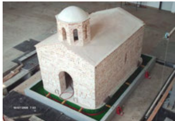
Fig. 2. Seismic base isolation by “ALSCL” floating-sliding system- model of church, 1/3.5
